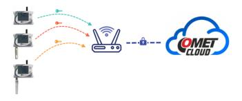
COMET WiFi sensors send data into COMET Cloud at selected interval via common 2.4 GHz WiFi infrastructure. WiFi sensors are equipped by own non-volatile memory for samples which cannot be sent in case of WiFi or ISP connectivity outage.
