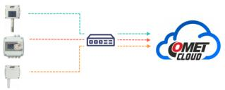
COMET Web sensors send data into COMET Cloud via Ethernet infrastructure. Measured values are sent via SOAP protocol transported by HTTP transfers. Authenticity of data transmission is done via unique entry point for each Web Sensor. This entry point is generated at COMET Cloud web interface and needs to be inserted to each Web Sensor separately. Authenticity of messages from Web sensors is secured when unique entry point is kept at secret.
