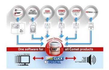
For customers which cannot use 3rd party Cloud service from the security reasons or users which want to execute data acquisition system at own server infrastructure is here COMET Database solution. COMET Database is a solution using Microsoft SQL database server as data storage and Viewer software installed at client stations.
