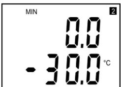
Press button again to display range and type of value for output 2 (symbol „2“). Here it is ambient temperature („°C“), when 0 V corresponds to -30 °C.
