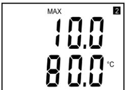
After next press of the button value for upper point appears, here 10 V corresponds to ambient temperature +80 °C. Press button again to end info mode and display actual measured values.
