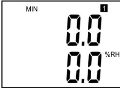
Range and type of value for output 1 (U<sub>out 1</sub> = symbol „1“ on display). Type of value, assigned to output 1, is indicated by displayed unit (here %RH = relative humidity). Upper line displays voltage value corresponding to measured value (lower line).
