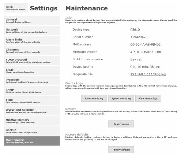
Network parameters are changed while you close jumper inside the device. After jumper closing it is necessary connect power supply. Factory defaults have no effect to user correction inside probe.
