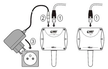
Web Sensor P8611 and P8641 connection (power supply adapter, Power over Ethernet):
