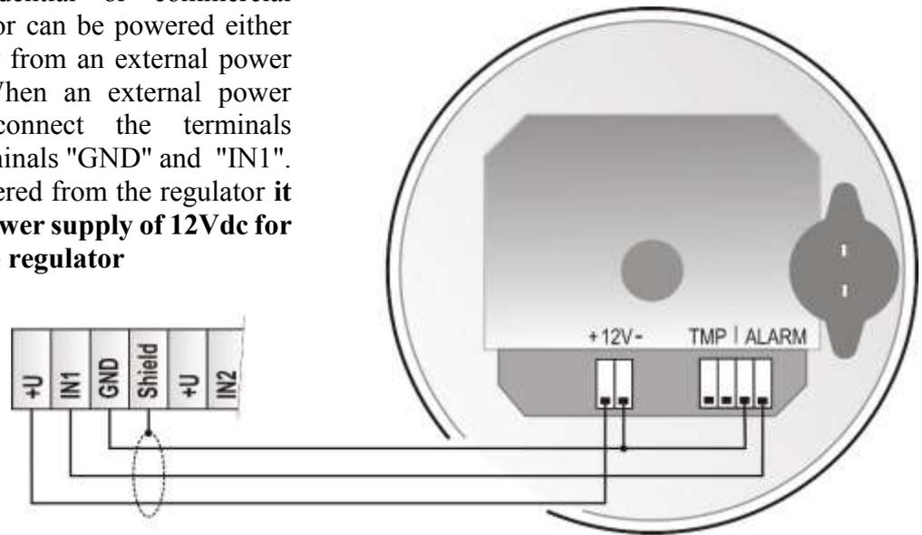
**Notice:** The connecting cables should be located as far as possible from the potential interference sources. The cable shield connect to "Shield" terminal of regulator only.
