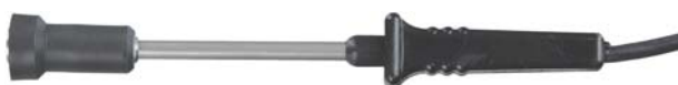
031-150/C - surface temperature probe -30 to +150 °C with Ni1000 sensor on 1meter cable for C3631, D3631 instruments
